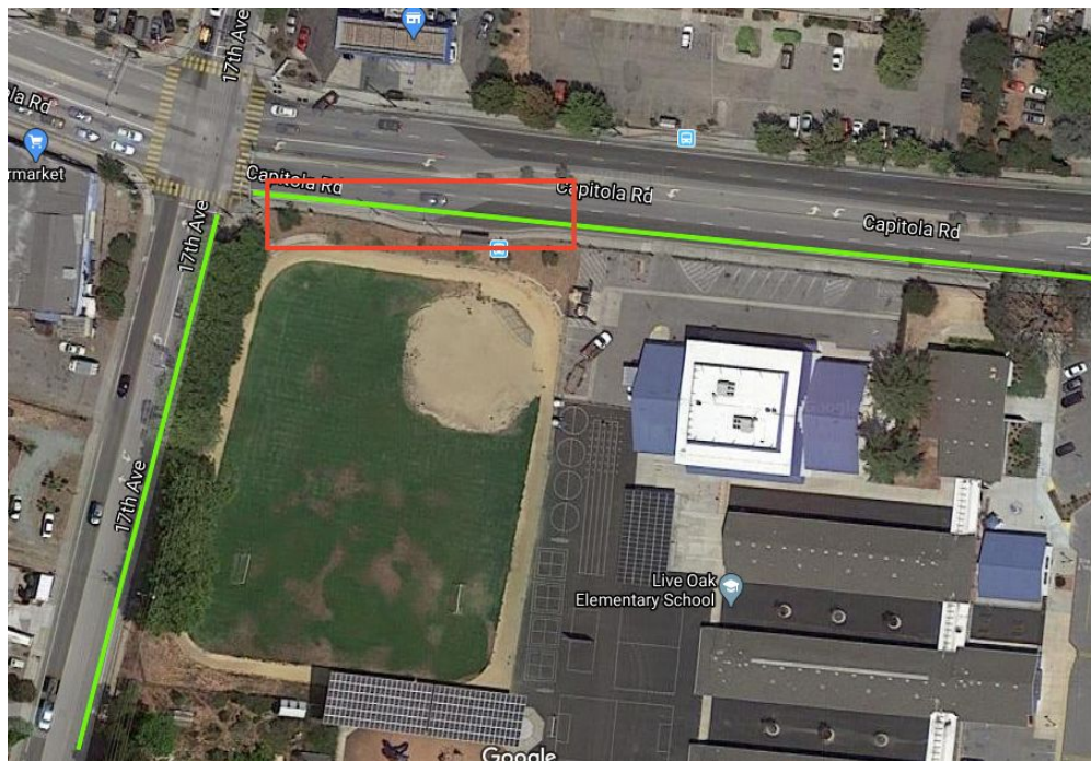
Figure 25. Two way bike lane along Capitola Road showing the connection from Capitola Road to 17th Avenue and highlighting the close-up image from figure 24 (red box).
