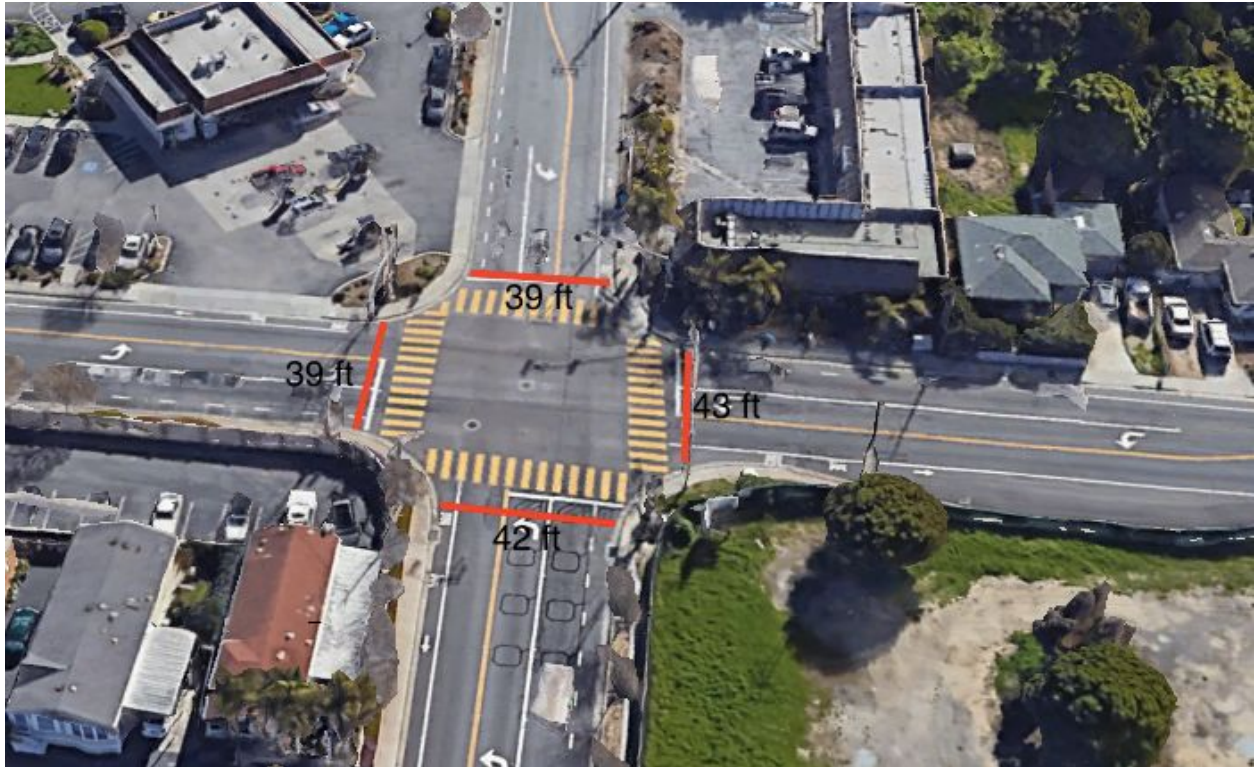
Figure 22. Aerial view of the current intersection at 17th Ave. and Brommer St. with the current dimensions
