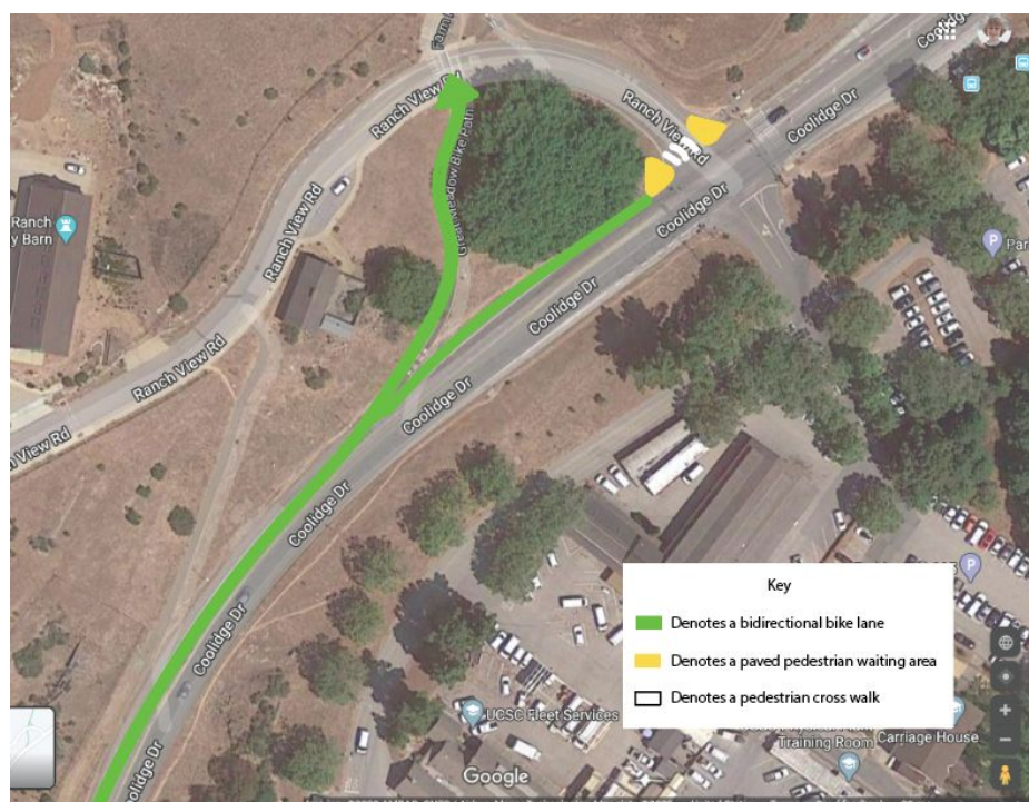
Figure 5.1.2: The placement of the bidirectional bikeway on Coolidge Dr. linking up to the Great Meadow Bike Path and including a crosswalk along Ranch View Road
