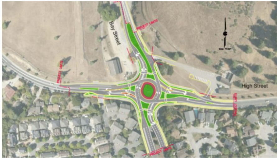
Figure 3.12.1. 2030 Roundabout Geometrics with improved crosswalks.
