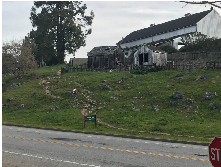
Figure 5.1.3: Desire lines along Coolidge Road due to lack of pedestrian infrastructure.
