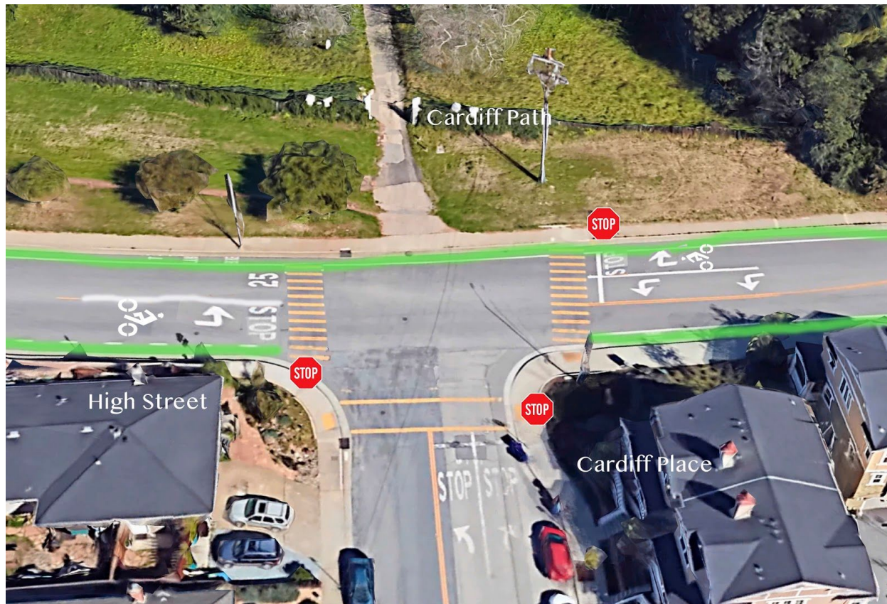
Figure 4.1.3: Intersection of Cardiff Place and High Street with additional stop signs and crosswalks.
