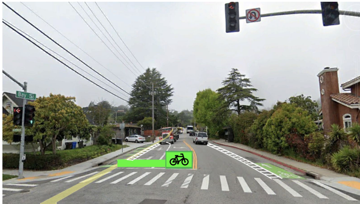
Figure 25 Proposed buffered bike lanes and bike box at the intersection of Bay & King
