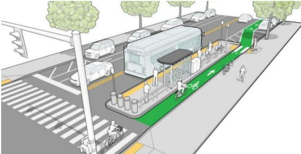
Fig 11. Floating Bus Stop Diagram Source (NACTO, 2014)
