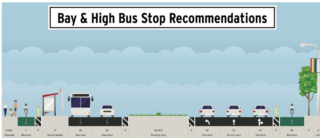
Figure 15 Recommended design with “road diet” and floating bus stops
