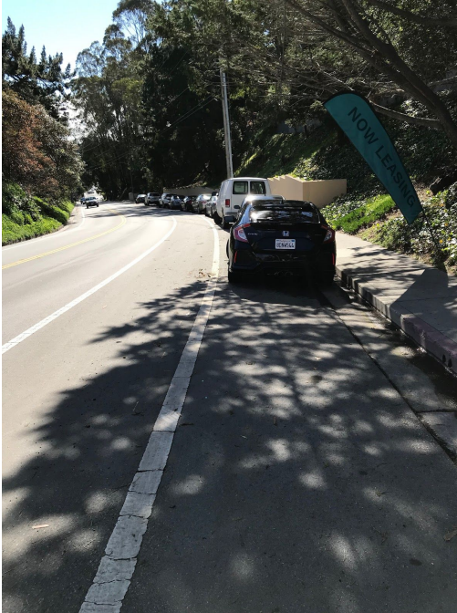
Bike lane along Western with high collision and dooring risk; Disappearing bike lane before a busy driveway
