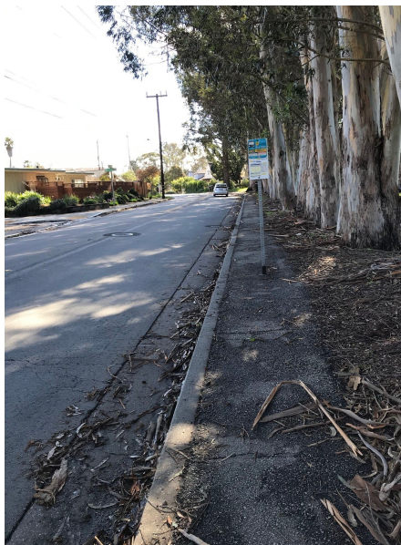
Bus stop in the middle of a single lane sharrow (i.e., no cutout)
