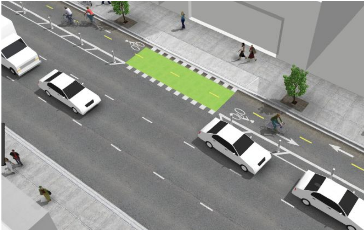
Figure 28: Detailed design for driveways along Water Street. Source: https://nacto.org/publication/urban-bikeway-design-guide/
