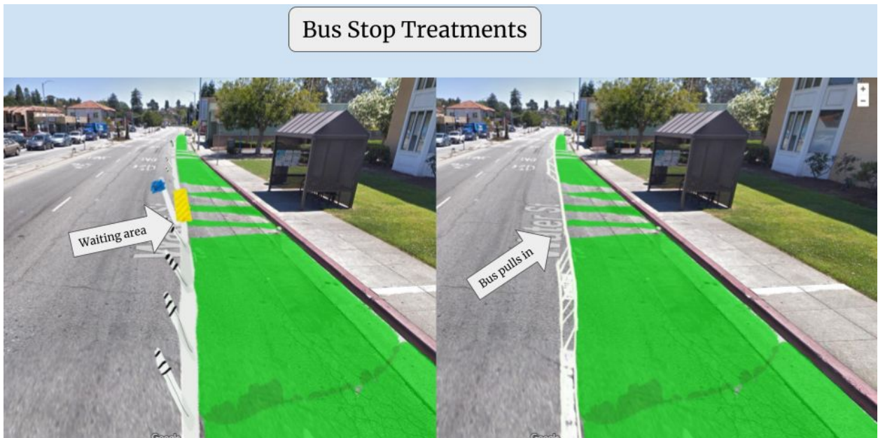
Figure 27: Detailed design for bus stops along Water Street. If there is adequate space, a waiting area/platform could be installed between the bike lane and the travel lane, as shown in the figure on the left. If not, passengers should wait in the shelter on the sidewalk and walk out to board the bus, as shown in the figure on the right.
