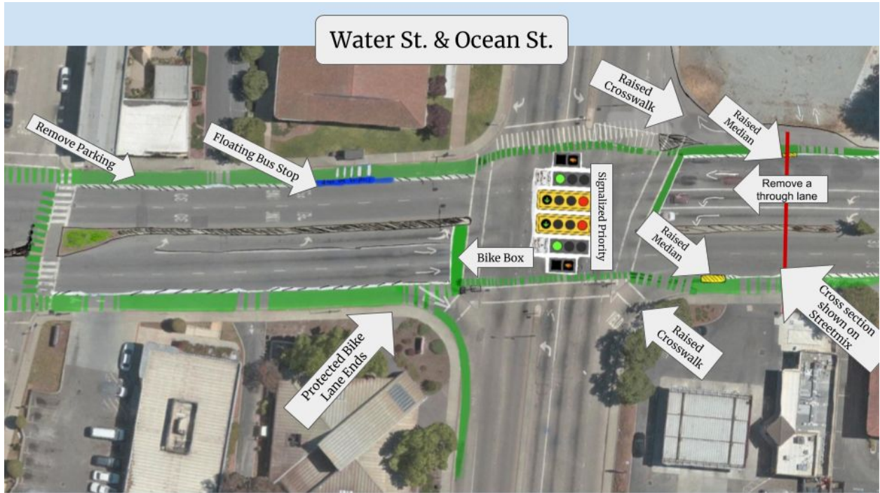
Figure 24: Aerial view of the new proposed designs for the intersection at Water Street and Ocean Street.
